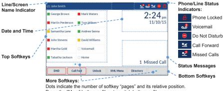
Dots indicate the number of softkey "pages" and its relative position. Press the "More" bottom softkey to switch bottom softkey pages. Swipe left and right in the top softkey area to switch top softkey pages.
